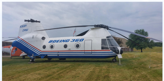
Boeing Model 360 (an all-composite, private venture, technology demonstrator)
